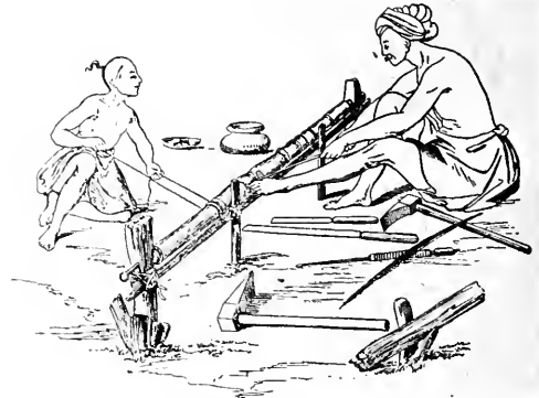
Fig. 10 AN ORIENTAL TURNER AND HELPER The helper drives the work by means of the wrapped cord or "belt." Note the "skill of toe" of the turner.
